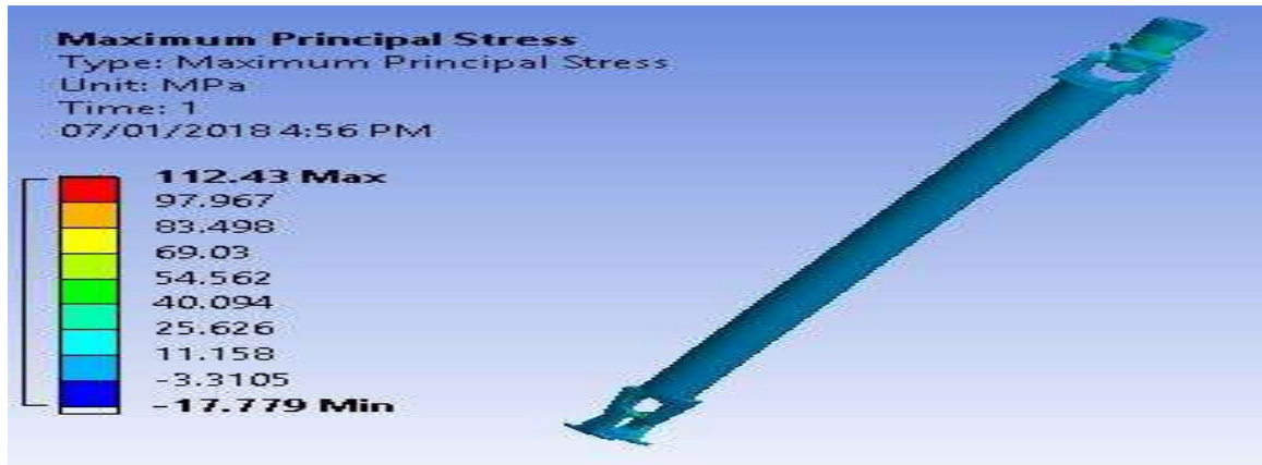
Fig. 4.2.1 Maximum Principal Stress for aluminium
