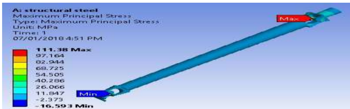
Fig. 4.2.2 Maximum Principal Stress for Structural steel
