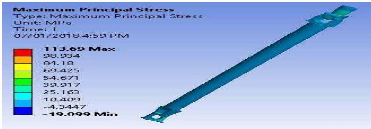
Fig. 4.2.3 Maximum Principal Stress for Titanium.
