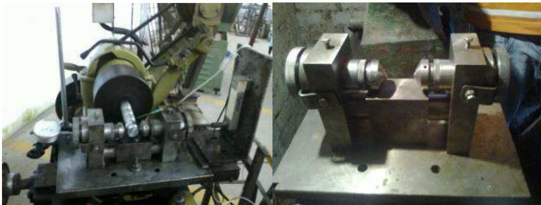
Fig 1: Fabricated Burnishing Tool using Lathe Machine
