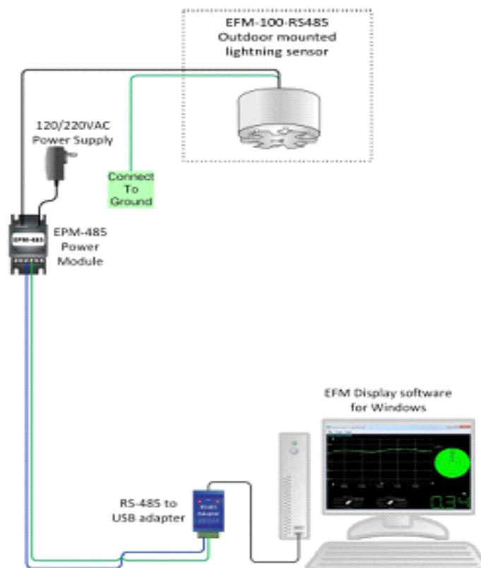
Figure 2 Block Diagram of Electric Field Mill.
