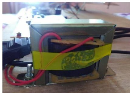
We use 12v and 5v power supply in our project. It is mainly used to provide DC voltage to the components on board. 5V is required for buzzer, LCD display, IR sensor microcontroller applied from power supply. And 12v is required for GSM module, motor.
