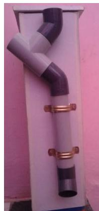
Pipe is connected to the floor of building. Garbage leave from pipe and this pipe is connected to the trolley. when bin is full then IR sensor sense, and send message to garbage van driver
