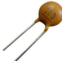
A ceramic capacitor is a fixed value capacitor in which ceramic material act as dielectric.
