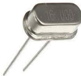
A crystal oscillator is an electronic oscillator circuit that uses mechanical resonance of a vibrating crystal to create an electrical signal. We use 11.0596MHz.
