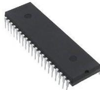
The AT89S52 is a low power high performance 8-bit microcontroller with 8K byte of flash programmable manufactured using Atmel's high density non-volatile memory technology. It is powerful microcontroller which provides a highly flexible and cost effective solution to many embedded control applications
