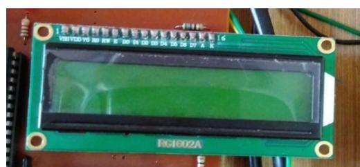
LCD (Liquid Crystal Display) is an electronic display. A 16\*2 and 24\*4 is very basic and commonly used in various devices and circuits. We used 16\*2 LCD display to show indication of “GABAGE BIN FULL”. We give 5v supply to LCD display.
