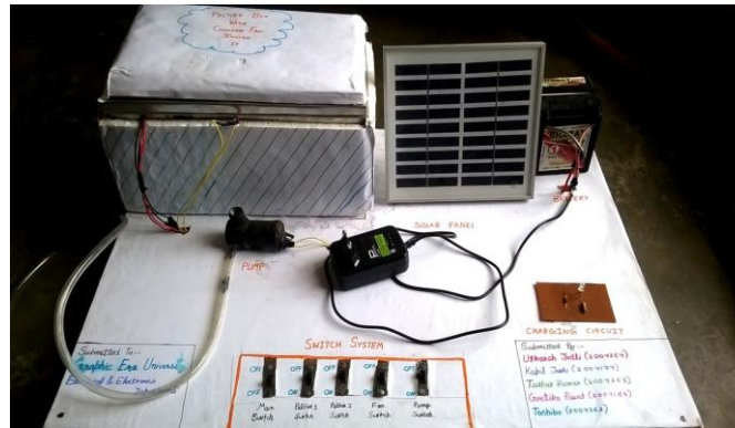
Fig. (2). Fully Developed Prototype of Solar Powered Air Conditioner.
