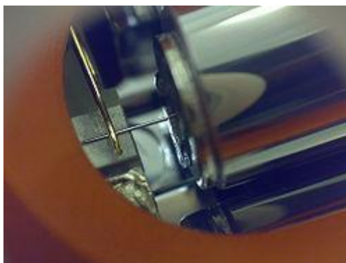
A close-up of a simple scanning tunneling microscope head using a platinum–iridium tip.
