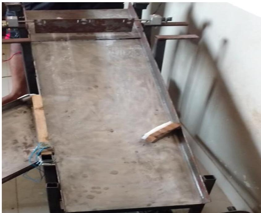
Conveyor system is common pieces of mechanical handling equipment that moves material from one location to another. We use the inclination conveyor system In that milk packages passes from start to end due to the inclination of the conveyer. Conveyors are especially useful in application involving the transportation of heavy
