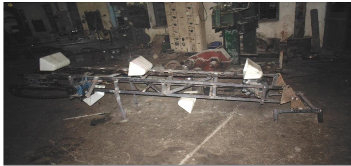
FIG.:3 actual setup of Solid Waste removal system
