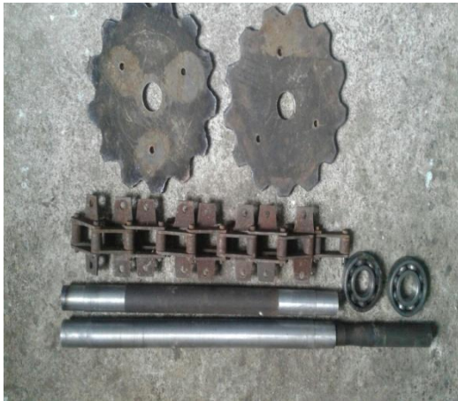
FIG.1 components of system
