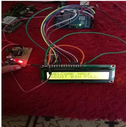
Fig. when Dustbin is full message is registered
