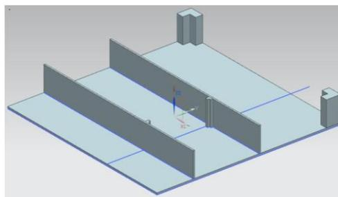
Fig.5.Fixture for heat sink mounting and holding the painting fixture
