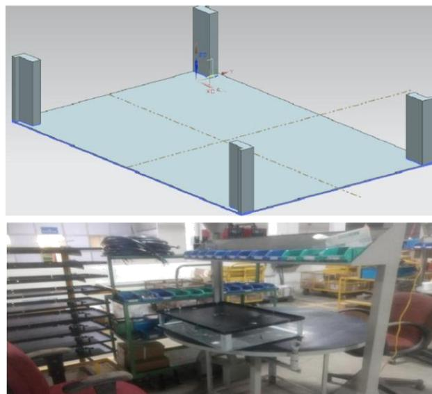
Fig.6.Fixture for holding tray
