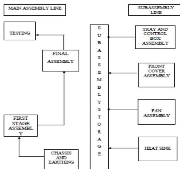
Fig. 1 The existing layout of assembly line
