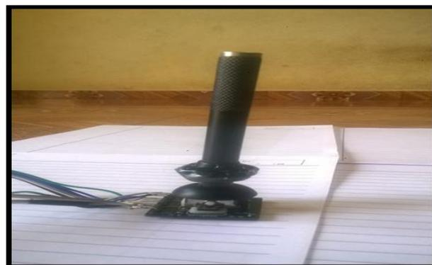
**Figure 8.2 :- Joystick Module(After Increasing Length)**
