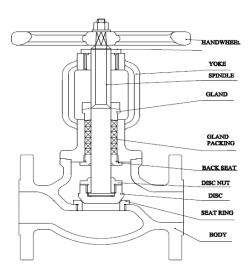
Fig.1.Diagram of Globe Valve body
