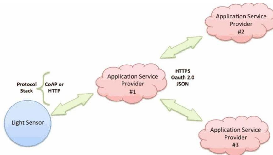
Figure 5. Back-end data sharing model diagram.
