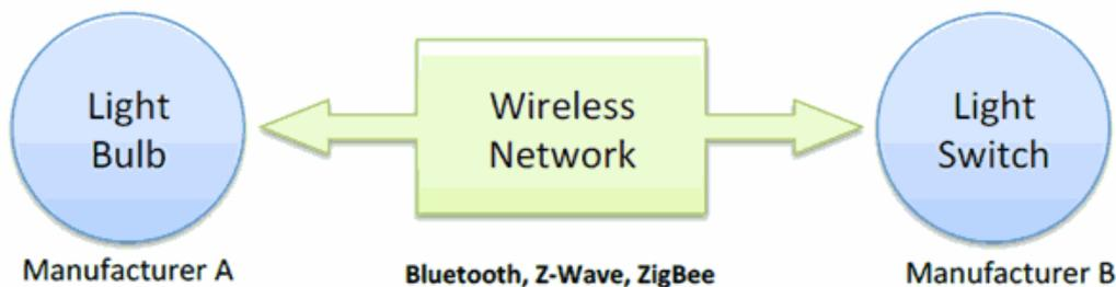
Figure 2. Device-to-device communication model diagram.
