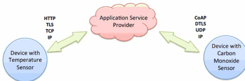
**Figure 3. Device-to-cloud communication model diagram.**
