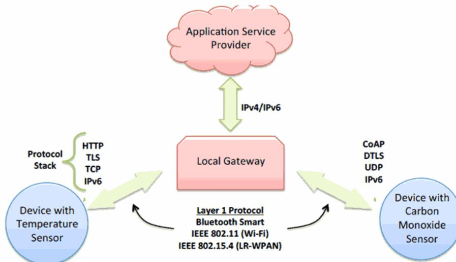
Figure 4. Device-to-gateway communication model diagram.
