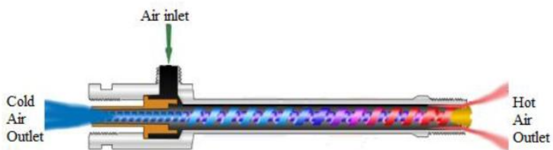
Fig. 1 Schematic Drawing of a Vortex Tube operational mechanism [2].
