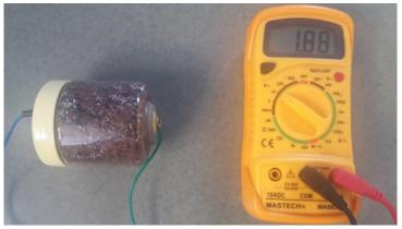
2) Around 3.75V produced with 2 MFC connected in series.
