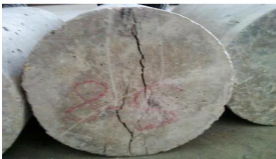
Fig. 3.2 Tensile testing of cylinder in CTM
