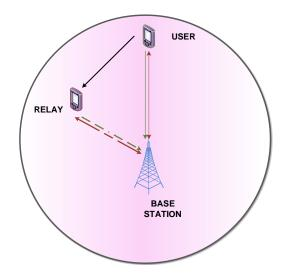
Fig.1. Relaying Devices with operator controlled link
