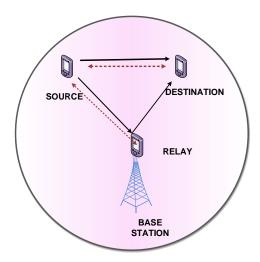
Fig. 3.Relaying device with device controlled link
