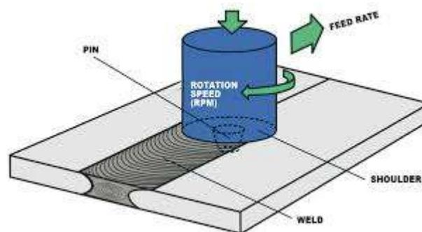
**Figure 1: Friction stir butt welding**
