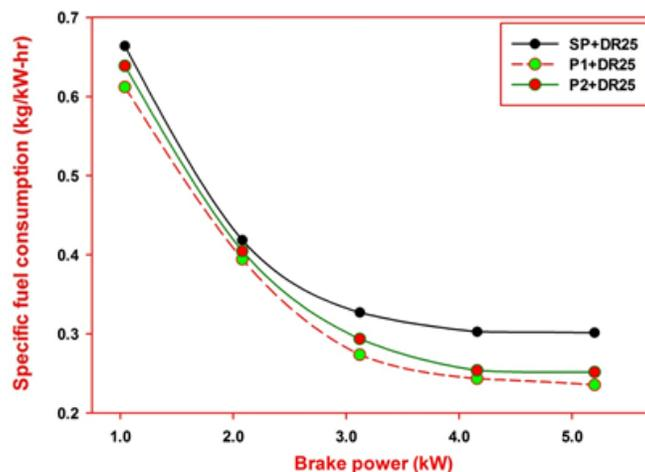
Figure 5. SFC using modified pistons with DR25 biodiesel blend
