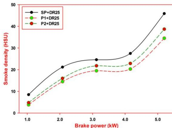
Figure 6. Smoke density using modified pistons with DR25
