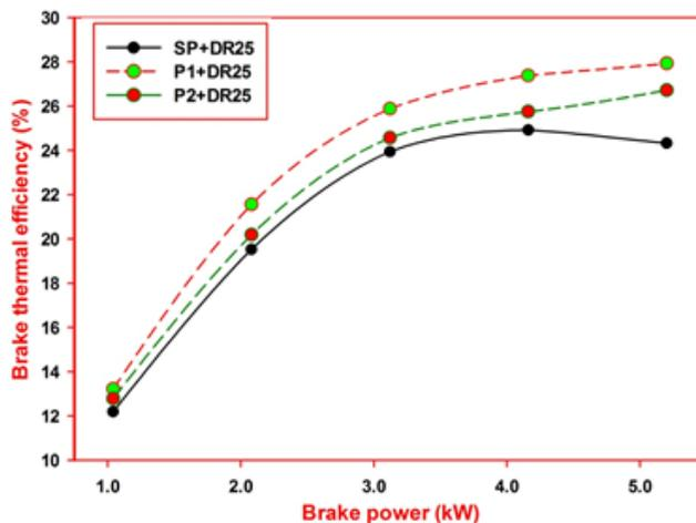
Figure 4. Brake thermal efficiency using modified pistons with DR25 biodiesel blend
