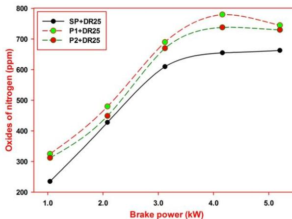
Figure 7. NOx emissions using modified pistons with DR25 biodiesel blend
