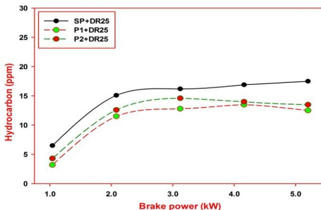
Figure 9. HC emissions using modified pistons with DR25 biodiesel blend
