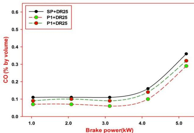
Figure 8. CO emissions using modified pistons with DR25 biodiesel blend
