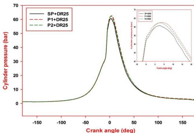
Figure 10. Cylinder pressure using modified Pistons with DR25 biodiesel blend
