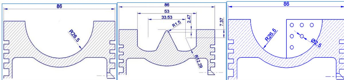
**Figure 1. Dimensions for standard piston (SP) (Left), Toroidal combustion chamber (TCC) (Center) and Swirl blade combustion chamber (SCC) (Right)**
