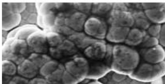
Figure 1: SEM micrograph of NiPZr (as-plated) EL nano-composite coated coupon
