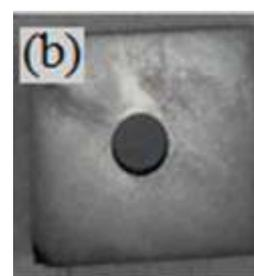
**Figure 3: Photographs after weight loss test of corroded coupon (a) NiPA as-plated (b) NiPZr as-plated**
