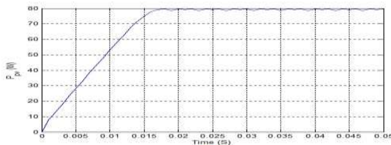
Fig.10: PV Power versus time curve produced by Perturb and Observe algorithm for step size of 0.7 and radiation of 1000 \text{ W/m}^2
