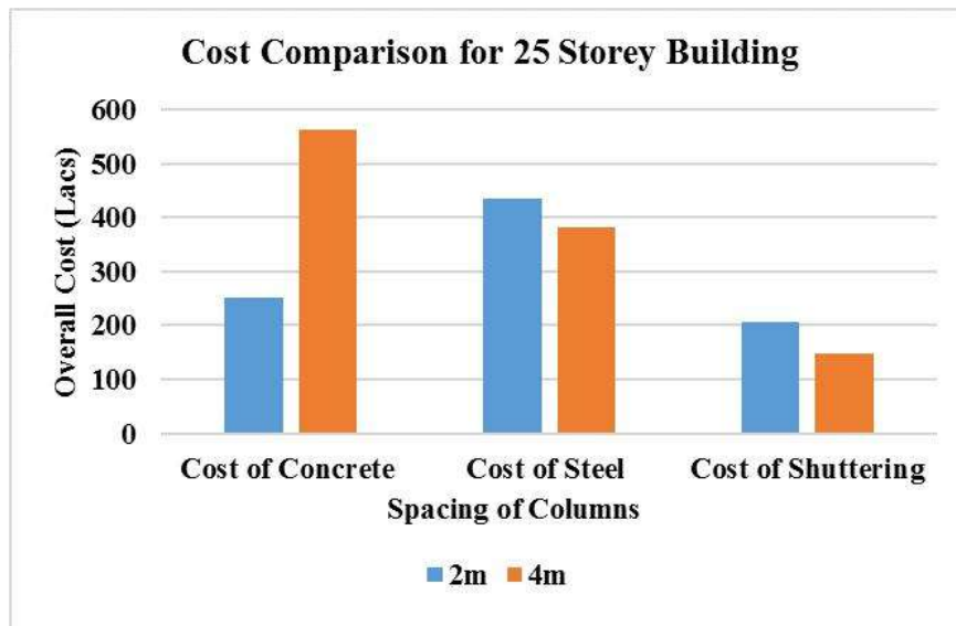
Fig. 3.1 Cost comparison for 25 storey building
