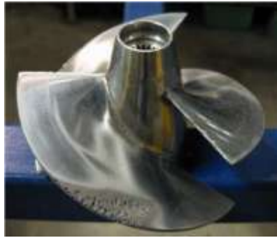
Fig. 3 damaged component due to cavitation
