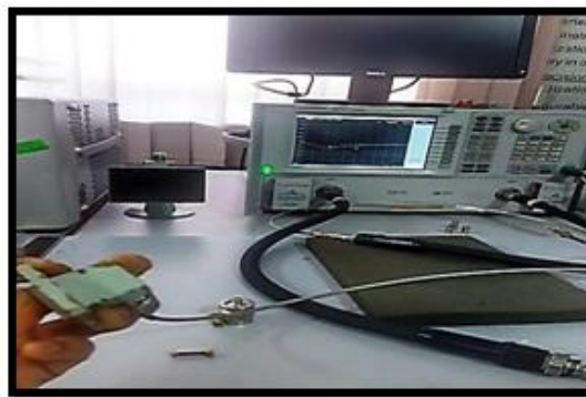
Fig. 8: electrical testing for reflection loss calculation, S_{11}
