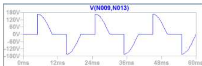
Fig. 11(a) Output voltage of (PCS) circuit at \alpha=90 deg
