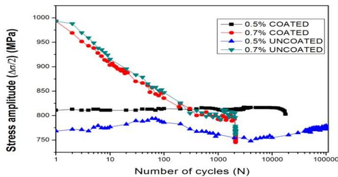
Fig 5: Cyclic stress response curves of alloy IN718 at 550<sup>0</sup>C for coated and uncoated samples
