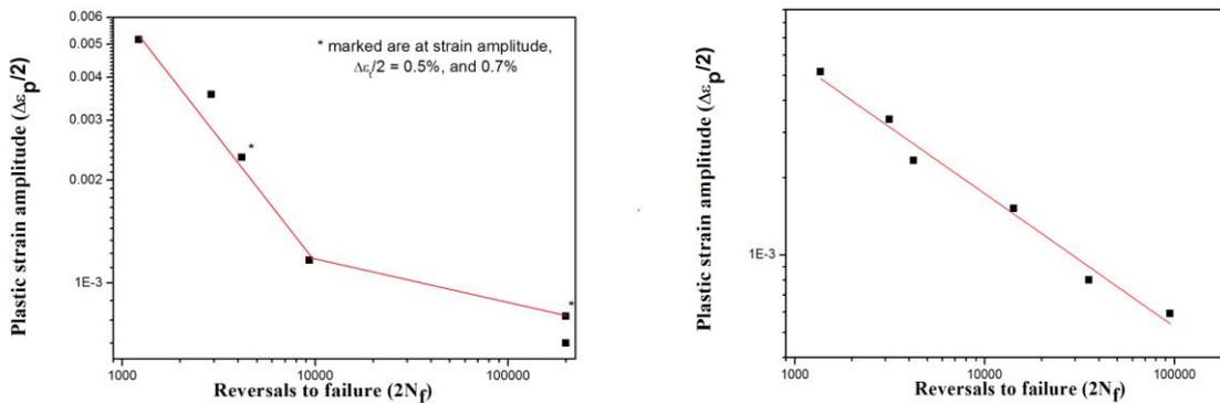
Fig 4: C-M plot (a) for uncoated sample at 550<sup>0</sup>C (b) for NaCl coated sample at 500<sup>0</sup>C [4]
