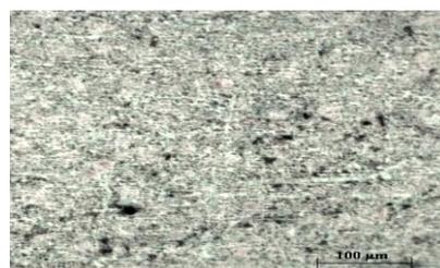
**Fig. 7: Optical image of cylindrical surface of the LCF uncoated sample tested at 550<sup>0</sup>C, (>10<sup>5</sup> cycles)**
