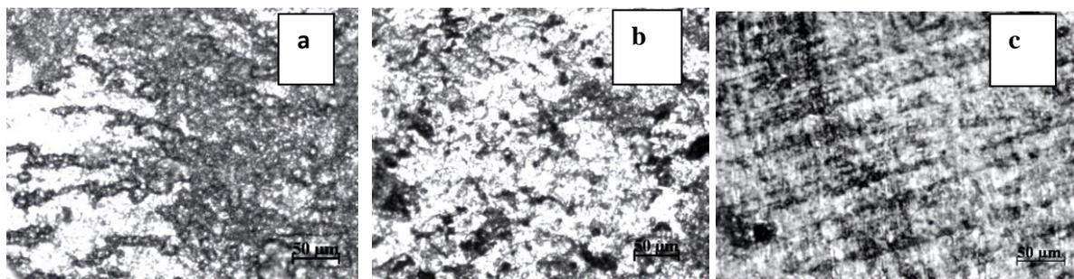
**Fig 6: Optical micrographs from cylindrical surface of LCF samples tested at 550<sup>0</sup>C, (a & b) NaCl coated samples, (c) uncoated sample.**
