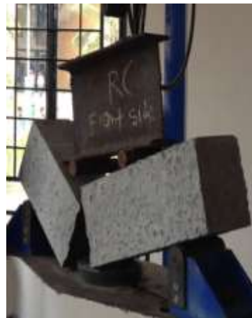
Fig 9: Flexural test on Beam
