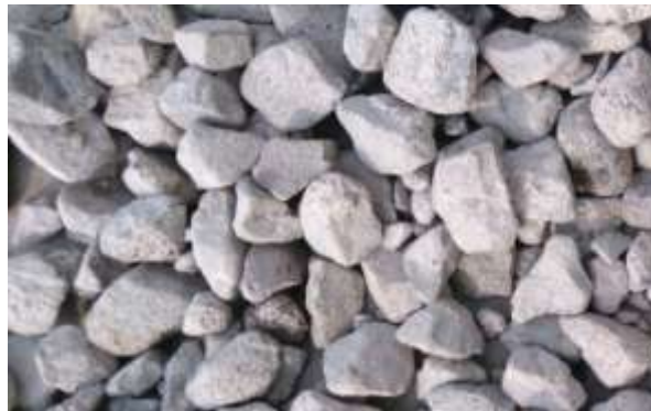
Fig 4: Recycled aggregates for 500 revolutions
