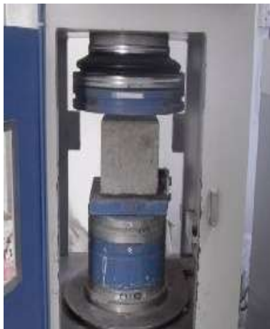
Fig 8: Compression test on Cube
