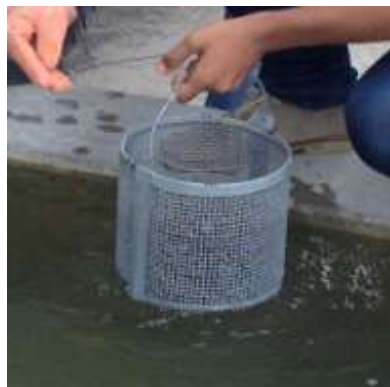
Fig 5: Washing of Aggregates
