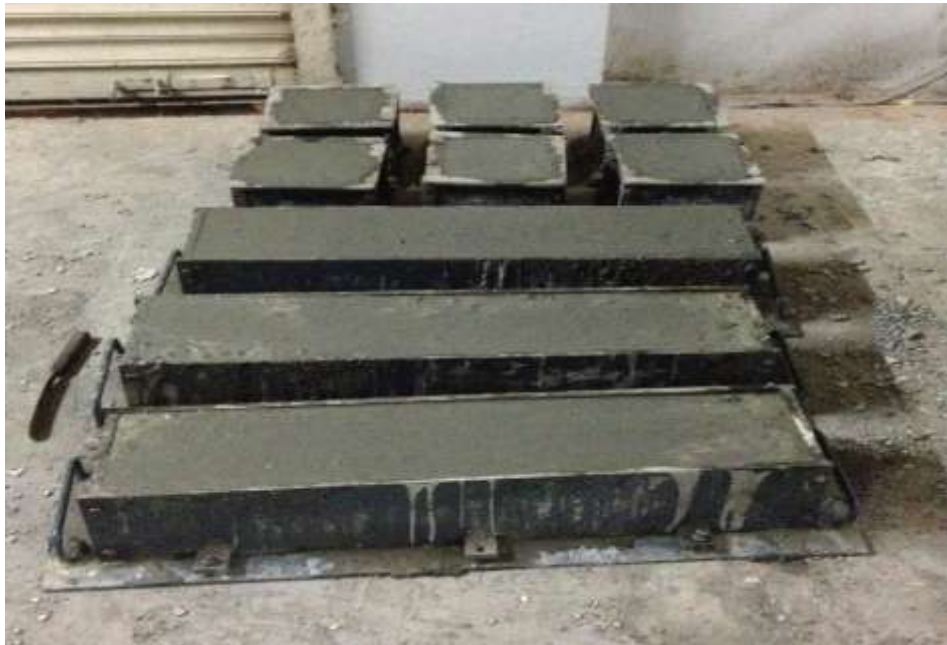
Fig 7: Casted Cubes and Beams
