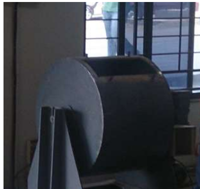
Fig 1: Abrasion Testing Machine
