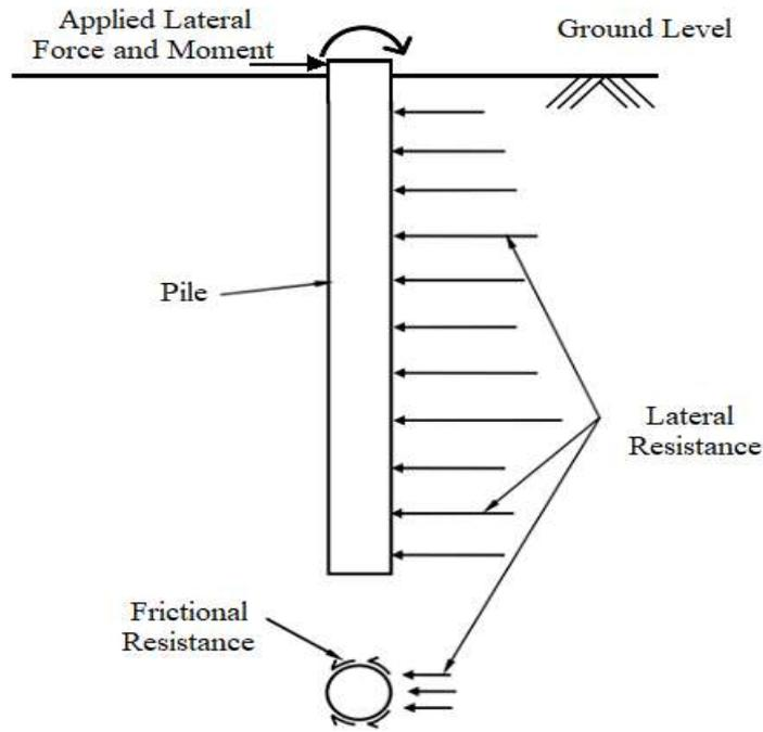
soil resistance acting over the entire pile shaft. Similarly, pile groups designed for horizontal load also have two resistance mechanisms i.e. friction along the sides and base resistance.
