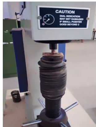
Fig 3.Specimen loaded at Rockwell Hardness testing machine
