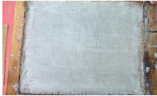
Fig.1.(b) Nanocomposites by Hand- layup technique
