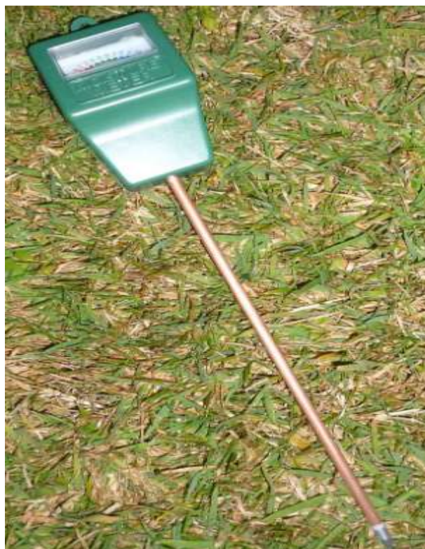
Figure 5. Soil moisture sensors
