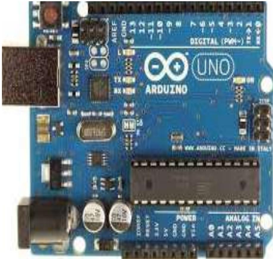
Fig.3 Arduino circuit
