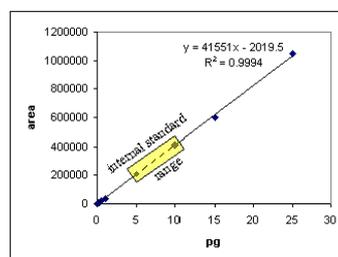
In this method, an internal standard is selected. Its known amount is added to the sample. It is not essential that the internal standard element should not be present in the original sample because this would not allow our knowing the total amount present.
