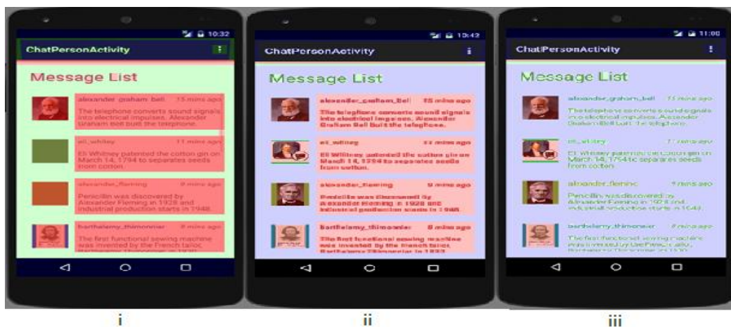
Figure 1: Removing the background to minimize overdraw
