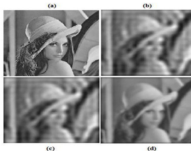
Fig. 3. Results obtained by Lowpass filters. (a) Original Image (b) Ideal LPF (c) Butterworth LPF (d) Gaussian LPF
