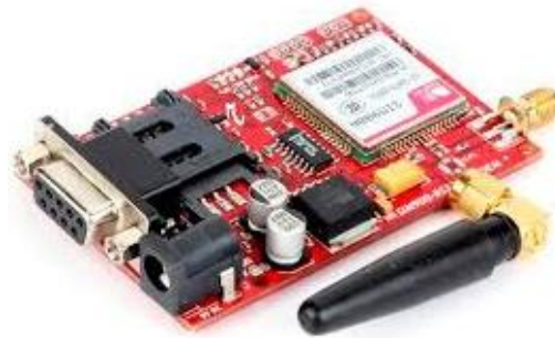
Fig 2.2: Global System for Mobile communications
