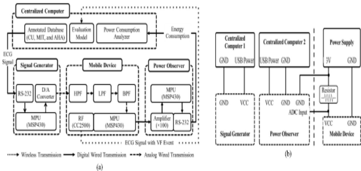
Fig 2. a) Block diagram of testing environment b) pin connection of the integrated sensing devices
