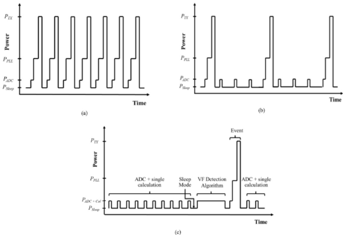
Fig .1. The conceptual graphs basecon the state transition for the three types of operations
