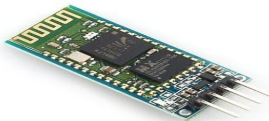
Fig.7.HC 05 serial port Bluetooth module
