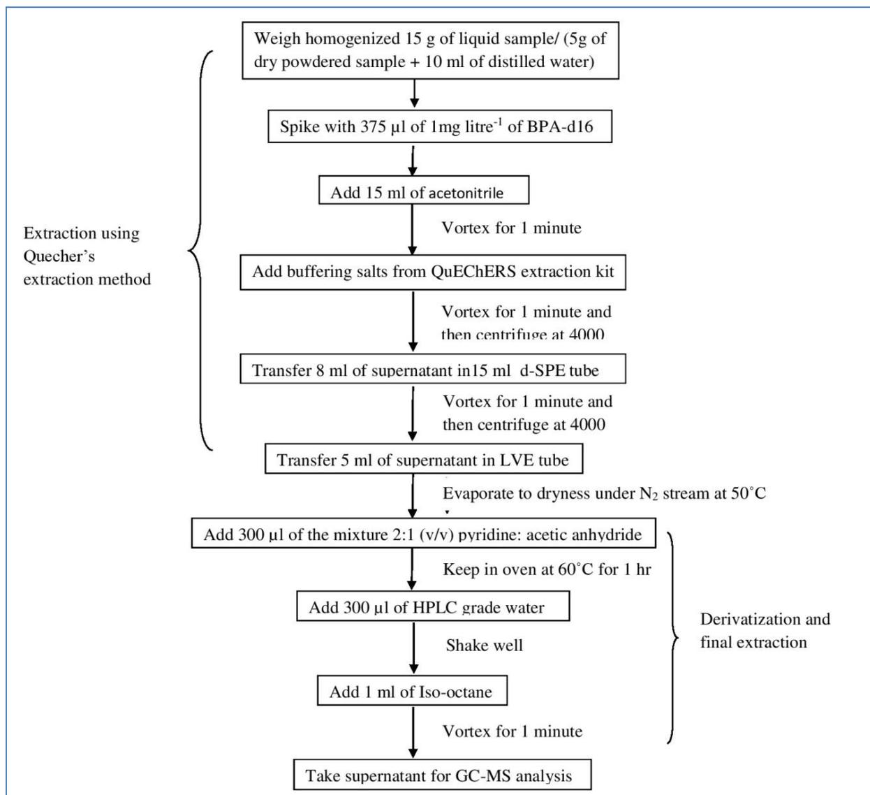
Fig.1 Scheme of sample preparation for BPA analysis
