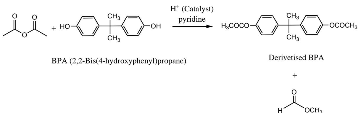
The one pot derivatization method followed by polarity based simple liquid-liquid extraction provided good yield, prevented loss of analyte and improved detection of BPA using Single Ion Monitoring (SIM) mode of single quadrupole GC-MS technique. The method was subjected to method validation in terms of sensitivity, linearity using internal standard calibration, limits of detection (LOD) and quantification (LOQ), accuracy and spiking study.
