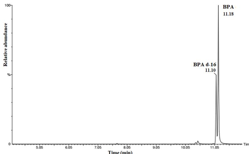
**Fig.3 (a) TIC of std solution of 25 ng g<sup>-1</sup> of BPA-d16 & 25 ng g<sup>-1</sup> using 5 channels (213, 224, 228, 270 and 312) m/z**
