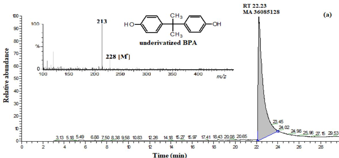
Fig.2 (a) Total Ion Chromatogram (TIC) of underivatized BPA 100 ppm std solution (along with full mass spectra of derivatized BPA at R 22.23)
