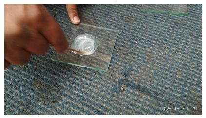
3. Mix both the solution and place other glass on it. Spread the solution evenly between surfaces.
