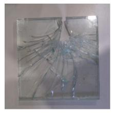
Installing Shatterproof glass can be very costly. But by this method it can be done in very low cost. Even if it does not provide security, it can prevent you against injury. The glass does not break into granules. It develops only cracks.
