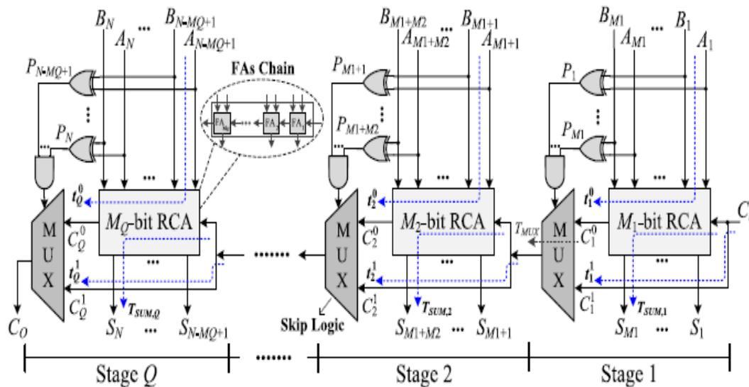
Fig. 1. standard structure of the CSKA
