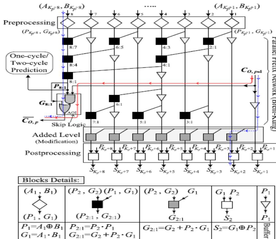
Fig. 3. Internal structure of the pth stage of the proposed hybrid variable latency CSKA
