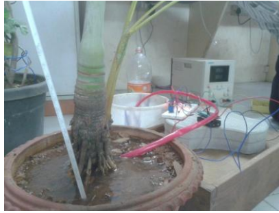
Fig 4. Trial Setup for Dry soil checking utilizing Mote
