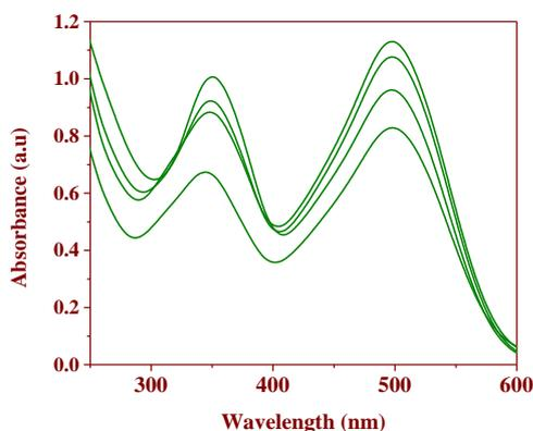
Fig.4 Absorbance spectrum showing photocatalytic degradation of Congo Red
