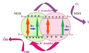
Fig.5 Mechanism suggested in the case of Photocatalytic degradation process using M1O/M2O (CuO/NiO)
