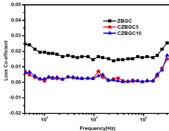
Fig.4.b. The Loss co-efficient of  $30$  ZnO-  $10\text{CuO}$ -  $60\text{B}_2\text{O}_3$  glass ceramics crystallized at  $775^\circ\text{C}$ .
