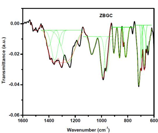
Fig.3.a. The Deconvoluted FT-IR spectra of  $40$  ZnO-  $60\text{B}_2\text{O}_3$  glass ceramics crystallized at  $775^\circ\text{C}$ .
