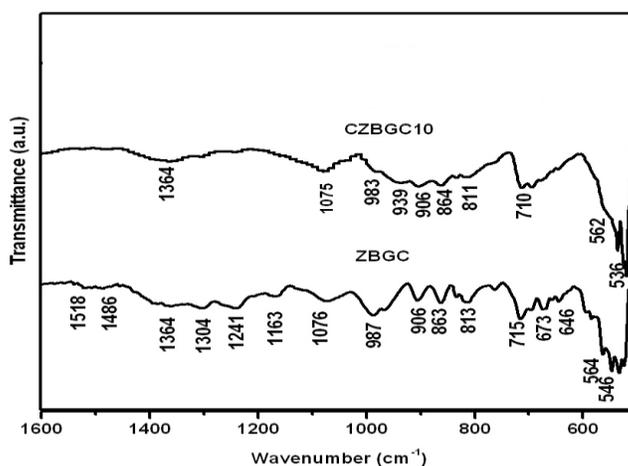
Fig.2. The FT-IR spectra of  $(40-x)$  ZnO-  $x$ CuO -  $60\text{B}_2\text{O}_3$  ( $x=0, 10\text{mol}\%$ ) glass ceramics crystallized at  $775^\circ\text{C}$ .
