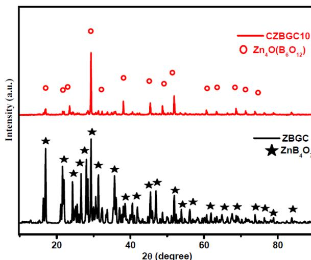
Fig.1. The XRD patterns of (40-x)ZnO-xCuO-60B<sub>2</sub>O<sub>3</sub> (x = 0, 10 mol%) glass ceramics
