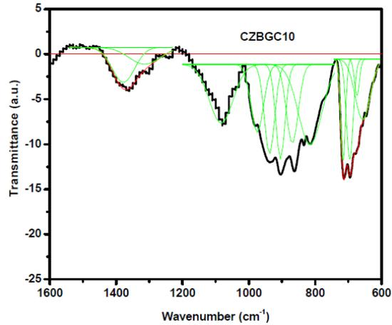
Fig.3.b. The Deconvoluted FT-IR spectra of  $30$  ZnO-  $10\text{CuO}$ -  $60\text{B}_2\text{O}_3$  glass ceramics crystallized at  $775^\circ\text{C}$ .
