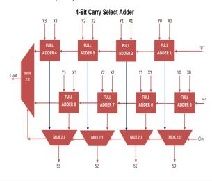
The linear carry select adder implies a particular way to implement the adder function. There are two results that can be calculated from the correct sum Cs which is taken and they are correct carry in, Cin and correct carry out Cout signals. So the delay the block size is calculated as  $(\sqrt{n})$ .
