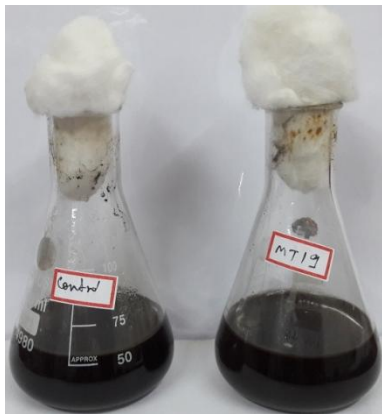
Fig 6 showing left flask as control without fungus and right flask MT 19 containing BH broth, fungal isolates, 0.1 % (v/v) Tween 80, 1% (v/v) crude oil and redox reagent (2% 2, 6- dichlorophenol indophenols) before biodegradation
