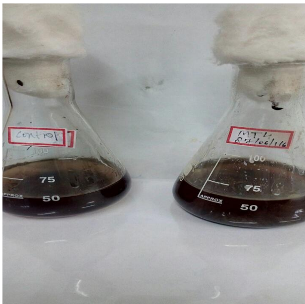
Fig 4 showing left flask as control without fungus containing BH broth, fungal isolates, 0.1 % (v/v) Tween 80, 1% (v/v) crude oil and redox reagent (2% 2, 6- dichlorophenol indophenols)
