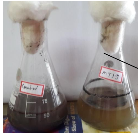
Fig 6 showing left flask as control without fungus and right flask MT 19 containing BH broth, fungal isolates, 0.1 % (v/v) Tween 80, 1% (v/v) crude oil and redox reagent (2% 2, 6- dichlorophenol indophenols) before biodegradation
