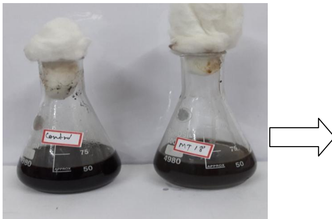
Fig 5 showing left flask as control without fungus and right flask MT 18 containing BH broth, fungal isolates, 0.1 % (v/v) Tween 80, 1% (v/v) crude oil and redox reagent (2% 2, 6- dichlorophenol
