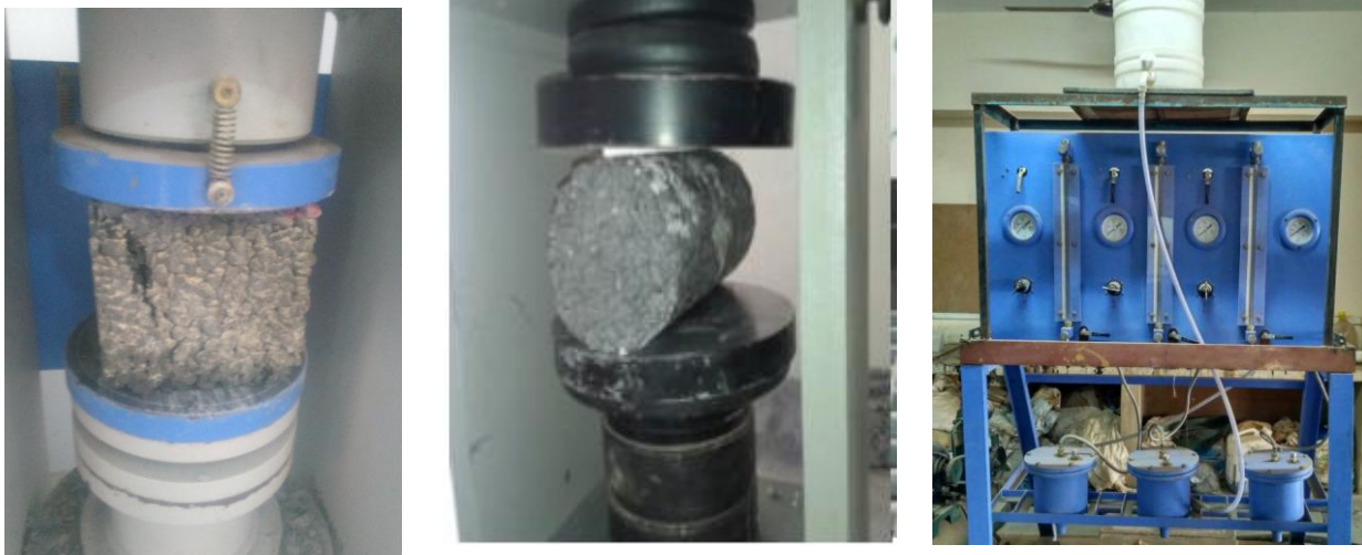
Figure 4.1 Compressive Strength, Split Tensile and Permeability Testing of Pervious Concrete specimen
