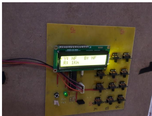
Fig.1 Single Line to Ground Fault Displayed on LCD
