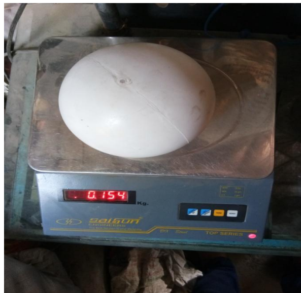
Fig. 5.1:- Measuring Weight of Hollow HDPE ball on Weighing Machine
