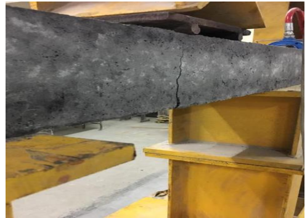
Fig.18: Deflected shape of the beam
