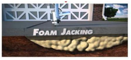
Figure 6: Raising of Concrete slab by Injection of Polyurethane Foam
